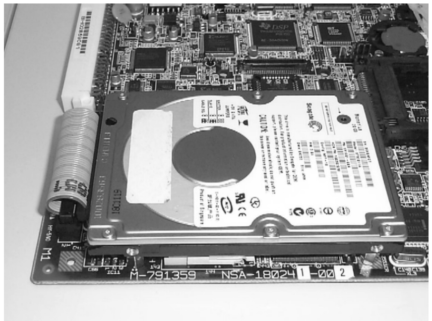
Figure 6-101 Placing the Hard Drive on the ETU
